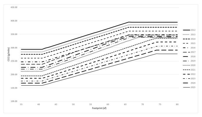
Figure I.2 CO<sub>2</sub> (g/mile) Light Truck Standards Curves
