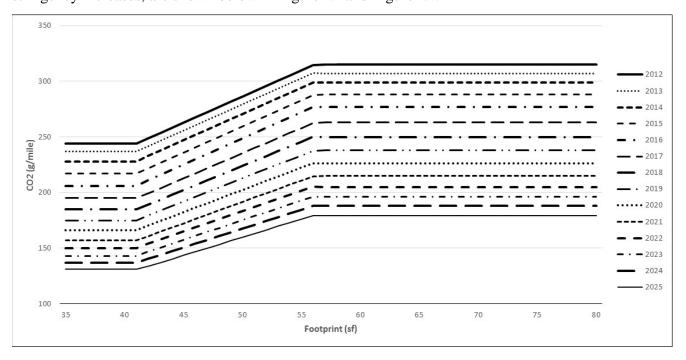
Figure I.1 CO<sub>2</sub> (g/mile) Passenger Car Standards Curves
